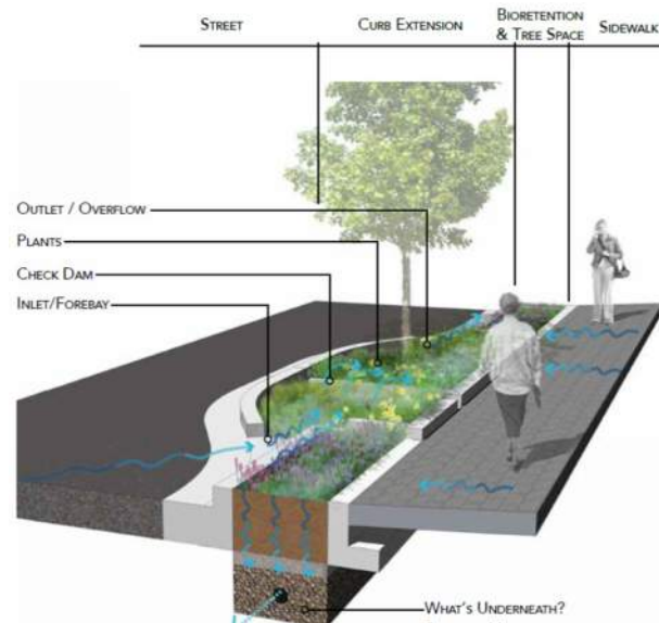
Indianapolis, IN (Cultural Trail): Bioretention bump outs in a R/W application to manage stormwater runoff from the street.
