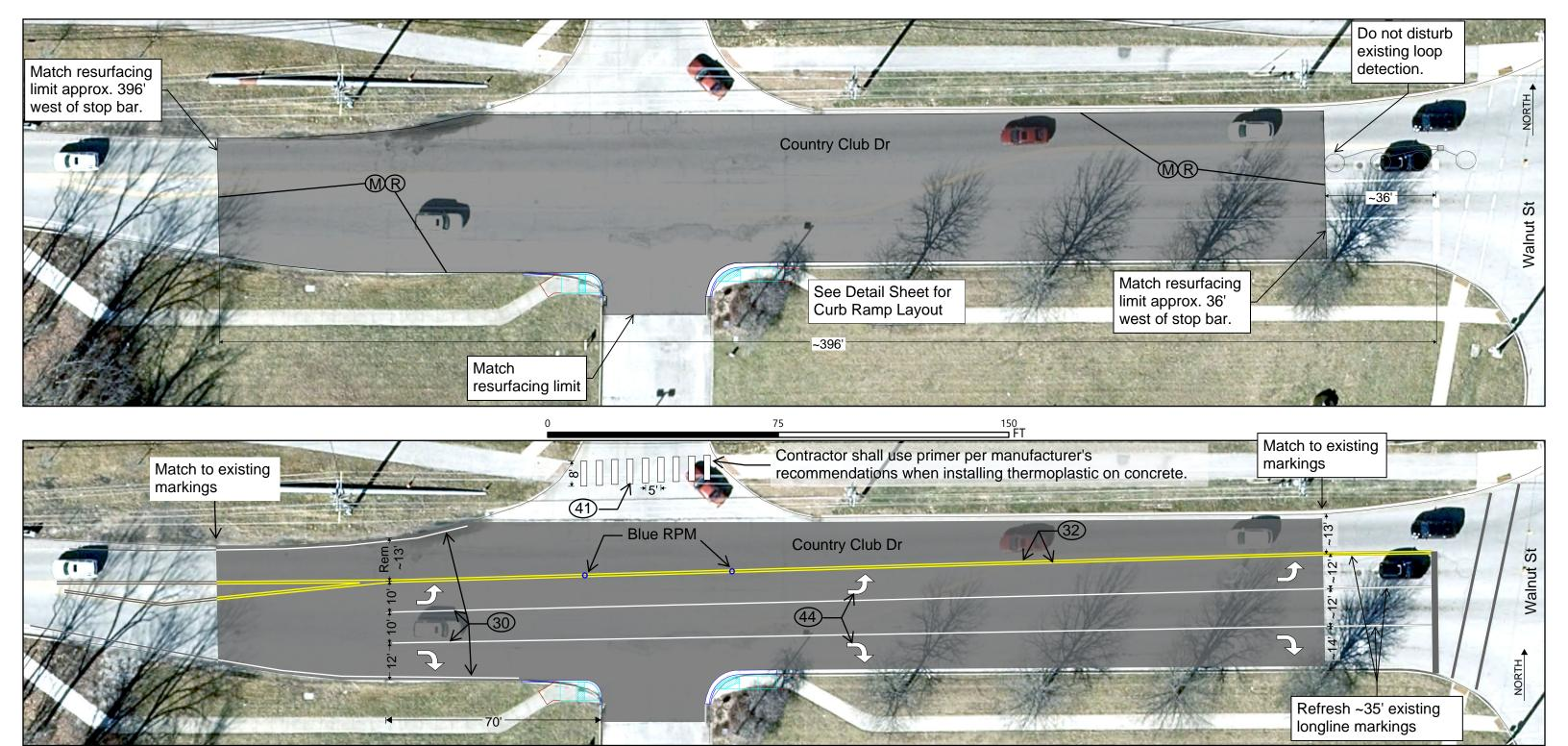
Note: 4 inch white edge line markings to be installed where indicated at 6 inches from edge of pavement.
