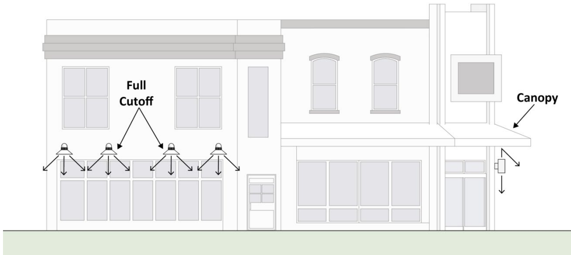
Figure 52: Exterior Light Shielding
