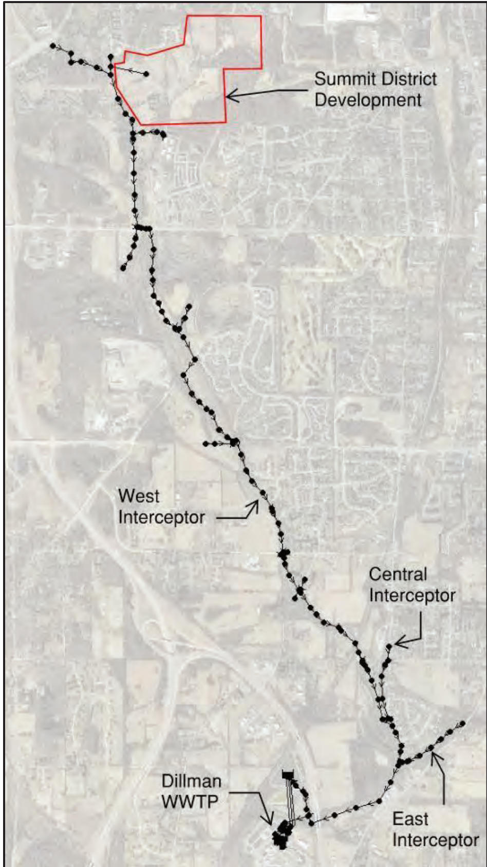
Figure 1-1: Dillman WWTP West Interceptor SWMM Hydraulic Model
