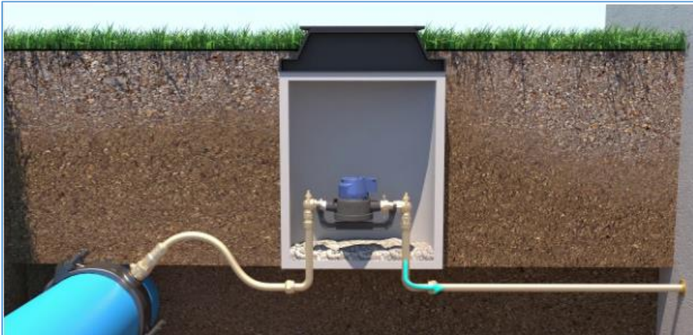
Example of a meter pit and service line set-up. Source: Mueller 2022.
