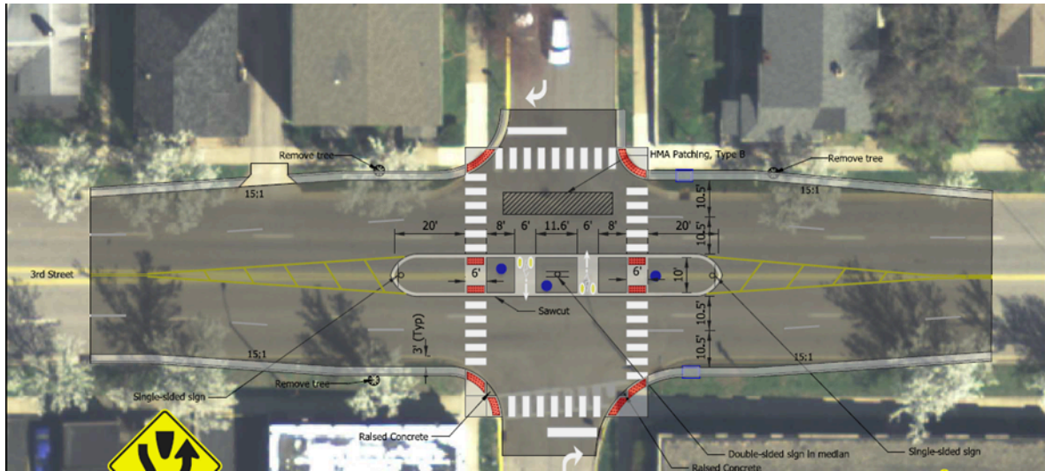
Above, Crosswalk Improvement Process project at 3rd and Grant Streets where new accessible curb ramps were installed.
