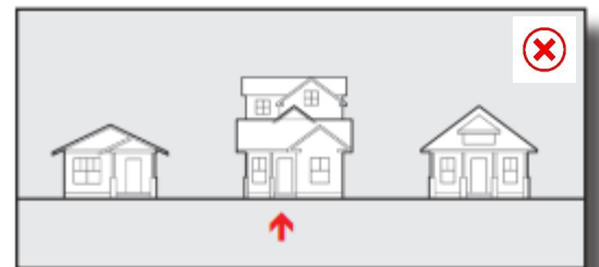
Incompatible addition; visually dominates original building
